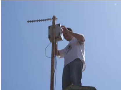
CRD scientist, Artur Reymers, establishing wireless connection of the geomagnetic sensors to CRD computers.
